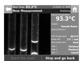
Once all of the sample capillaries are deemed to have finished, or the instrument reaches the previously specified end temperature, the instrument will complete the measurement and display the samples analysis report.
