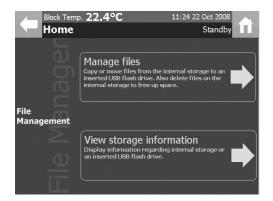
**Manage files:** Result files can be copied, moved or deleted from the devices internal storage.
