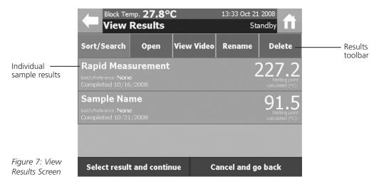
The View Results screen allows the user to perform a number of actions with the result files stored on the instrument. The actions available are displayed in the Results Toolbar.
