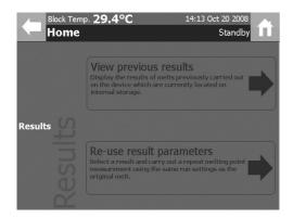
**View previous results:** Displays the result files of melt determinations previously carried out on the device which are currently located on internal storage.
