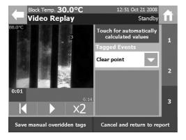
1 Select the capillary tube to which the manual event is to be added by pressing the relevant "Capillary selection" button.
