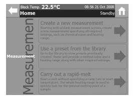
**Create a new measurement:** This option allows a new melt determination to be started. Measurement parameters such as the Sample Name, Start Temperature and Ramp Rate need to be entered when using this option.
