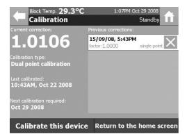
15 The calibration screen is now updated to show the new calibration details. The Calibration history window will now update to display details of the previous calibration.
