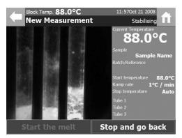
5 When the sample block reaches the start temperature the SMP40 status will change to "Stabilising" and the temperature of the sample block will remain constant for 60 seconds
