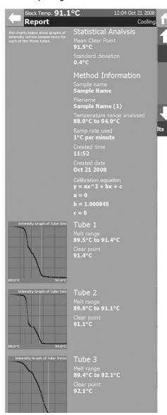
When a melt determination is complete or a result file is opened, the screen will display the Report Screen.
