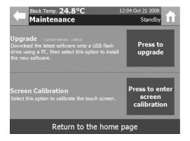
1 To upgrade the instruments software, firstly download the new software version onto a USB flash drive. Insert the USB flash drive into one of the SMP40's USB ports and touch the "Press to upgrade" button. The new software version will be automatically installed onto the instrument.
