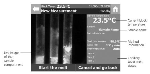
Figure 6: New Measurement Screen
