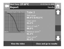
The melt determination report is updated with any manual events that are added and saved. An asterisk next to the event name is used to denote that it has been manually added by the user.
