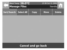
3 Once the move action has been completed the files will no longer be available on the instrument so ensure that no further reprocessing of the results is required before using the move action as it is not possible to move the file back, from the USB flash drive to the instrument, once the action is complete.
