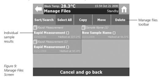
The View Results screen allows the user to perform a number of actions with the result files stored on the instrument. The actions available are displayed in the Result Toolbar:
