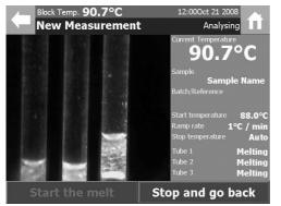
8 As the melt determination progresses the capillary tube melt status changes through:
