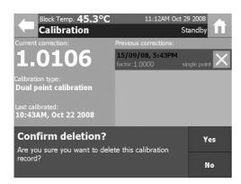
16 If a calibration record needs to be deleted, pressing the X next to the calibration record will display a confirm deletion dialogue box. Press "YES" to confirm or "NO" to cancel.
