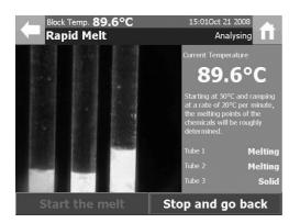
1 The rapid melt function will heat the sample from 50.0°C at 20.0°C/min until the sample has melted.
